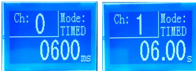
Figure 3 【TIMED】 type, and time unit is s & ms
